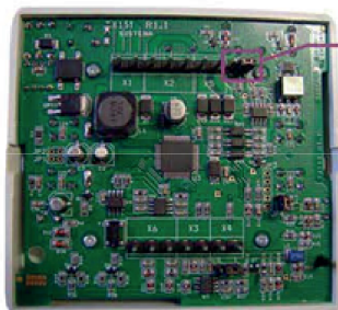
EOL resistor (JP6 pin block)
